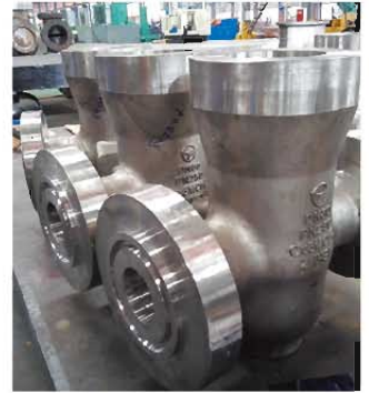
3" Class 1500 Self Sealing Slab Gate Valve
